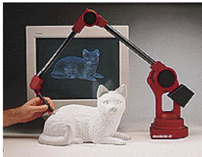
Figure 8.2. A 3D digitizer (courtesy Micro-Scribe)
