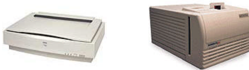
Figure 6.1. A flatbed scanner and a slide scanner
