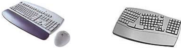
Figure 3. A standard (left) and a natural keyboard (right)
